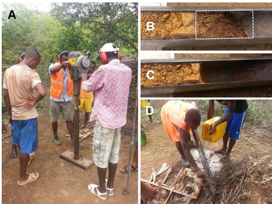
Figure 5-12 Window Sampler Demonstration
