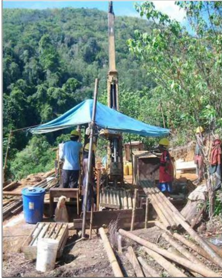
Figure 5-13 Photograph of the Versadrill Kmb.4km Drill Rig in Operation (Gilbertson, 2013)
