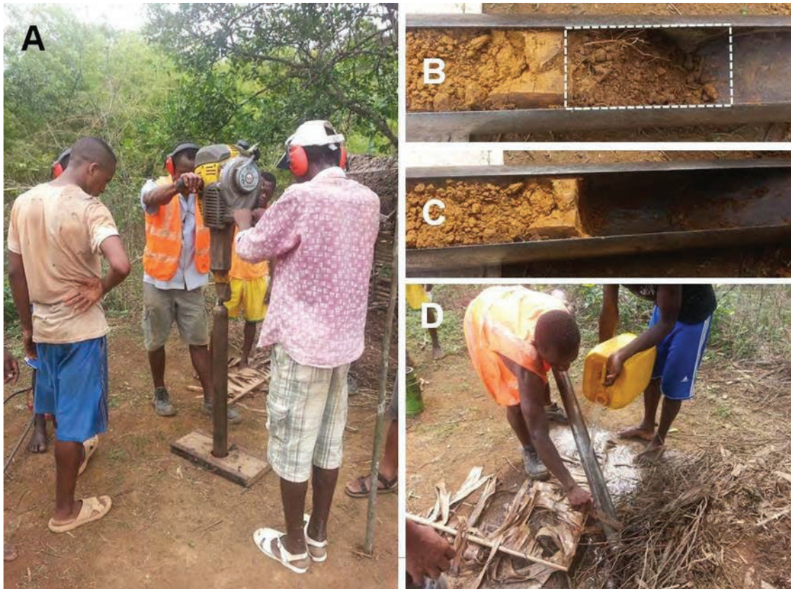
Note: A. Window sampler in action. B. Sample tube with fall back material from previous meter (in white box). C. Contaminated material removed. D. Cleaning of sample tube prior to next run.
