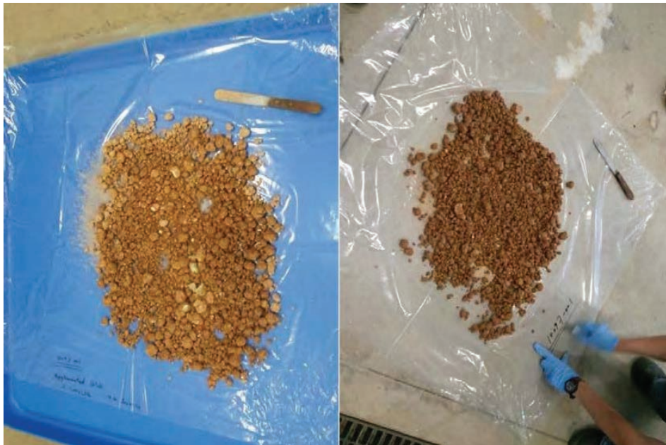
Figure 5-17 Column Tests Agglomerated Feed - Column 1 (left) and Column 2 (right)
