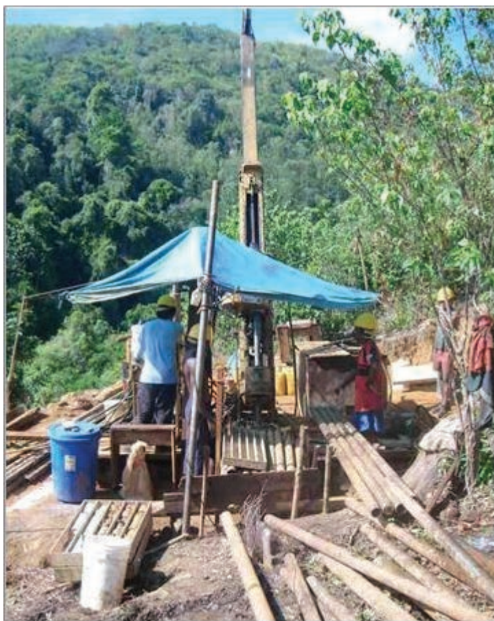
Figure 5-13 Photograph of the Versadrill Kmb.4km Drill Rig in Operation (Gilbertson, 2013)
